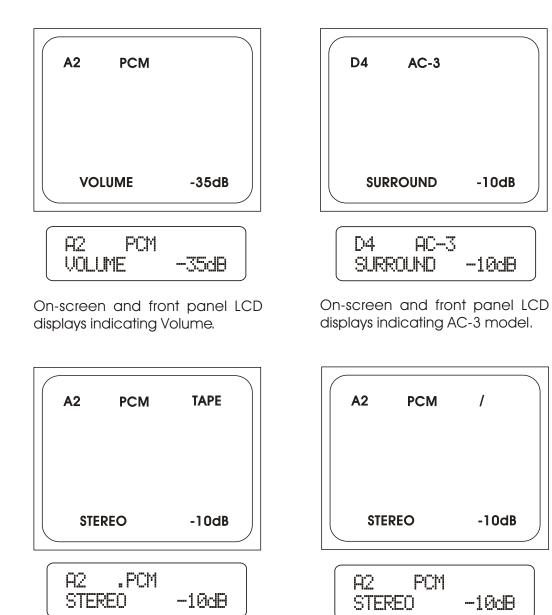
On-screen and front panel LCD displays indicating tape monitor on.
